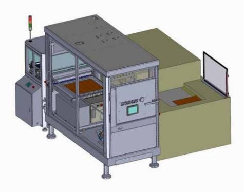
The V1-LDI Loader / Unloader was designed to load direct imaging machines drastically reducing human intervention. This machine medium designed to serve and prototype PCB shops with a large job mix. The V1 - LDI Loader has the capability to load and unload inner and outer layers with dry film, roller clean the top surface and lay them on the DI table to be exposed.
